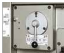
Power down feed 0.05, 0.1, 0.2 mm/rev
